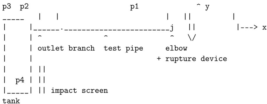
The experiment consists in a large tank filled with pressurized air (Initial pressure = 62 bar), its outlet branch being connected to the test pipe. The test pipe is a 3m-long and 50.8mm-diameter straight cantilever pipe with a 90° elbow at its extremity. Its free end is sealed with a rupture device. A protective plate is set near the tank where the pipe will impact when whipping.
