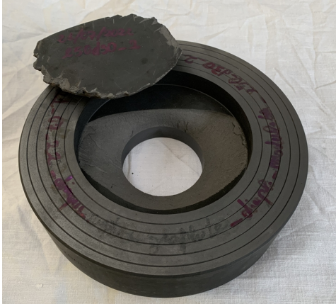
Figure: Graphite bursting disk and failure cone.
